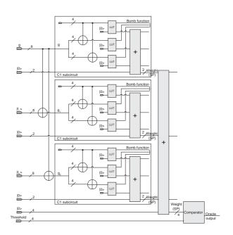
Figure 4. Four Variable Oracle Circuit
